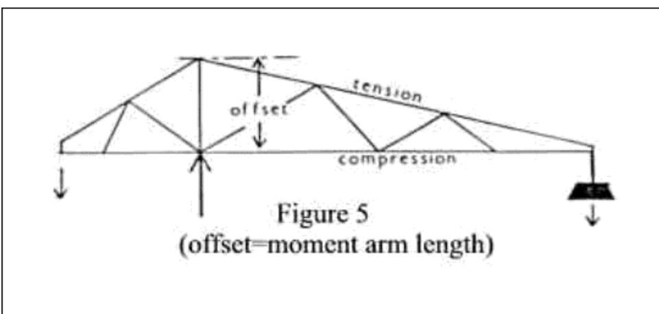
In evaluating the forces on the spine in lifting, the body must be seen as a cantilever like the jib of a crane (Figure 5) There is a compression component and a tension component and the offset between them is critical to the strength.
